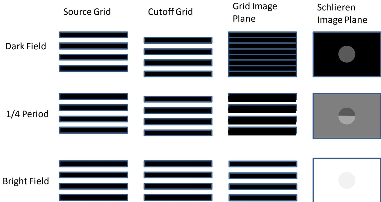
Figure 2. Effect of grid alignments for dark field (1/2 period shift), bipolar schlieren (1/4 period shift), and bright field (no shift) alignments.
