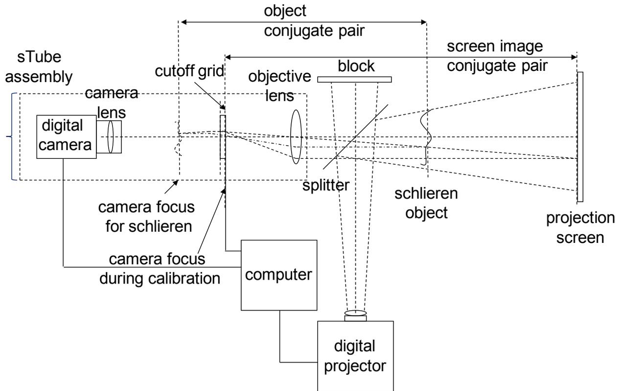
Figure 5. Digital projector based digital focusing schlieren system.
