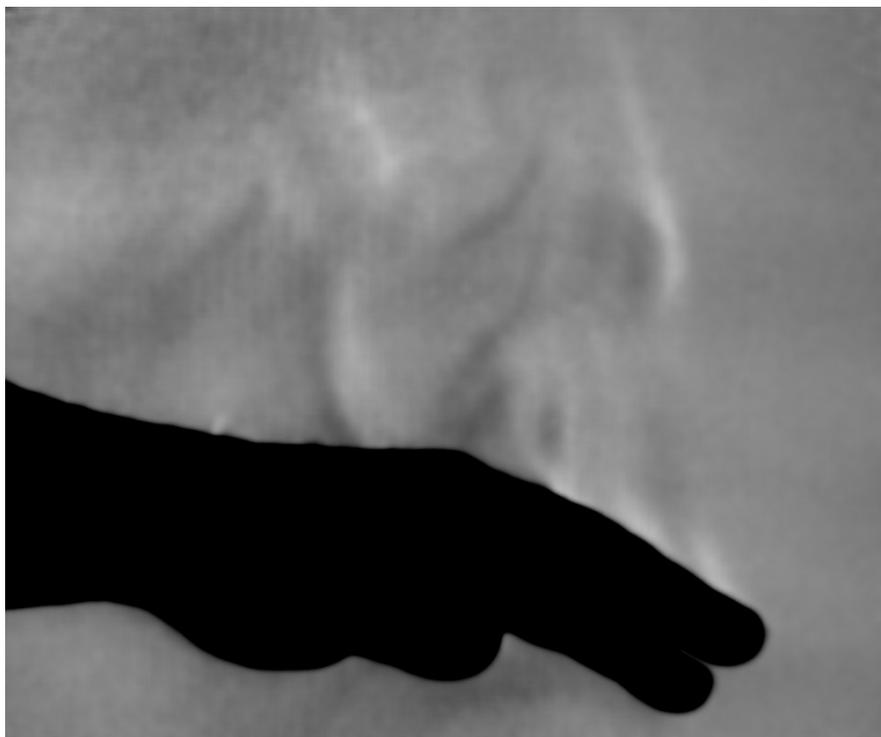
Figure 7. Closeup of schlieren image of experimenter's hand with body heat convection using an LCD television.
