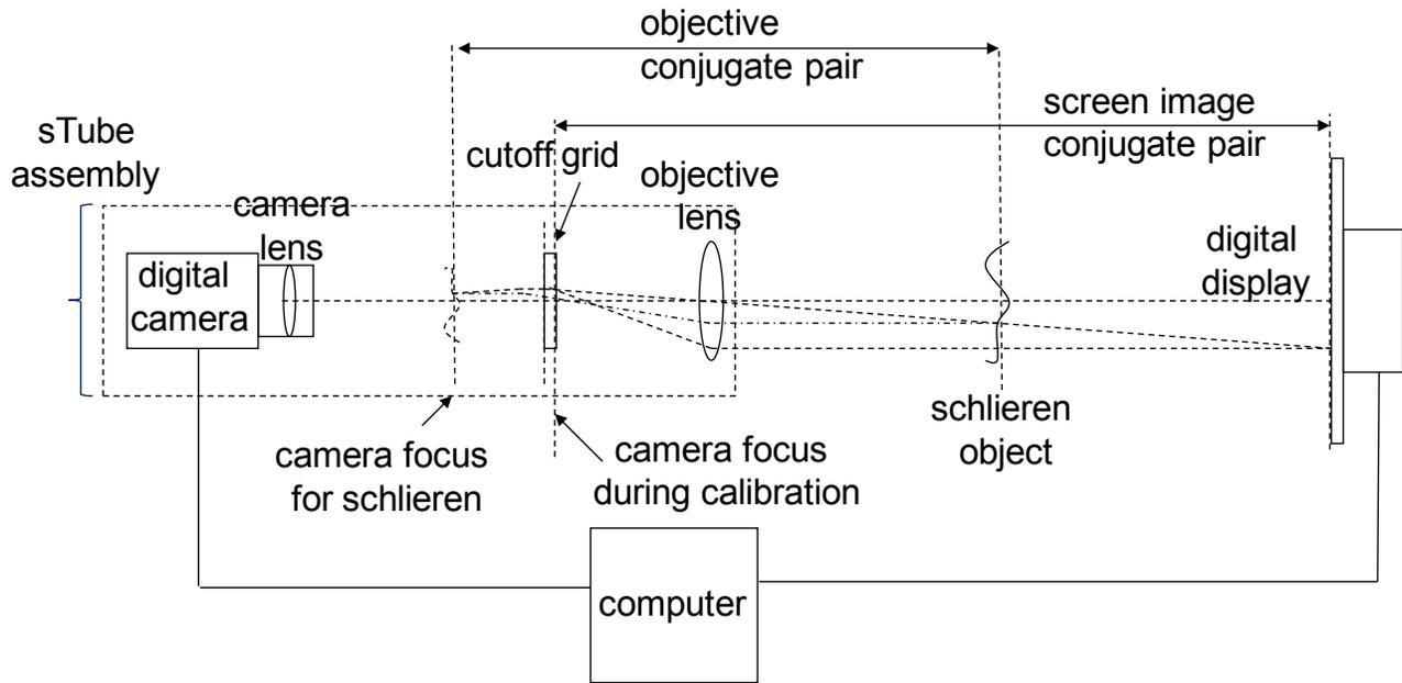
Figure 3. Backlit digital display based digital focusing schlieren system.
