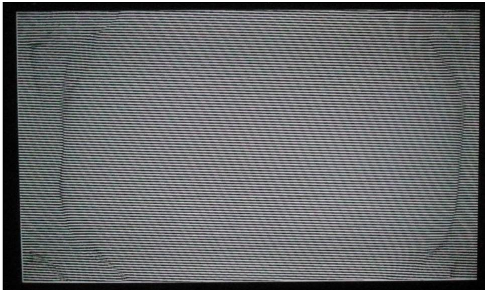
Figure 6. Complementary grid for an LCD television through a Ronchi ruling. Note distortions due to aberration near the edges.
