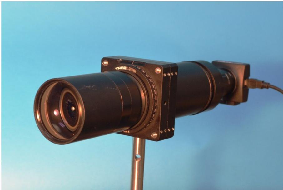
Figure 4. Cutoff filter mounted with receiving optics for use with a digital display.
