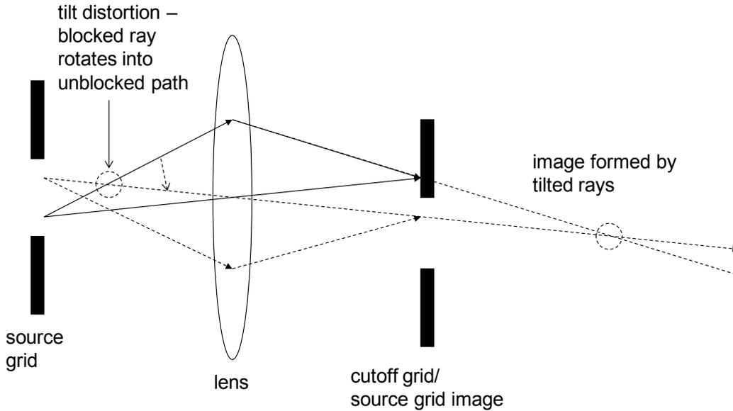
Figure 1. Diagram of focusing schlieren image formation.
